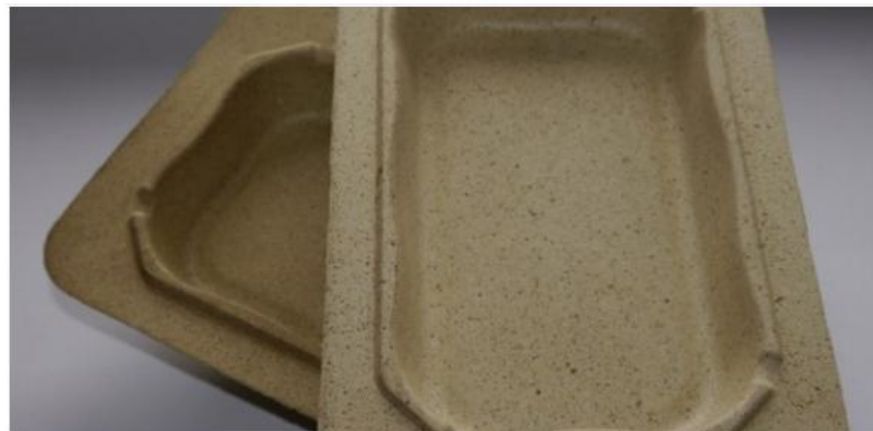
Trial mouldings are 250 x 150 x 50mm but different sizes will be offered
