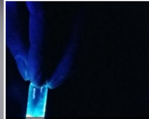
no-sizes 'carbon dots' that are used to make LEDs (credit: Prashant Sarswat)
